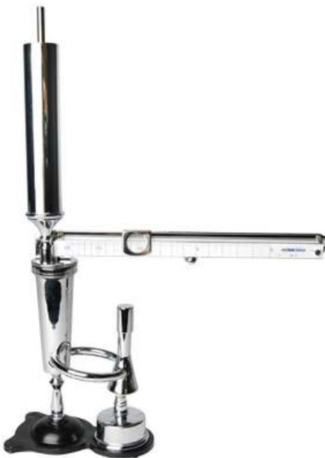
1. Fill the conical heater with water up to the bottom ring. This way, the thermometer (that needs to be screwed onto the heater) won't touch the water. The water level can easily be adjusted with a plastic pipette
